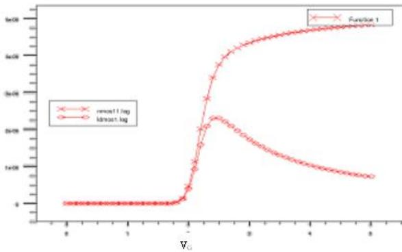
Fig. 3: Transconductance ( $g_m$ ) vs gate voltage ( $V_G$ ) curve.
