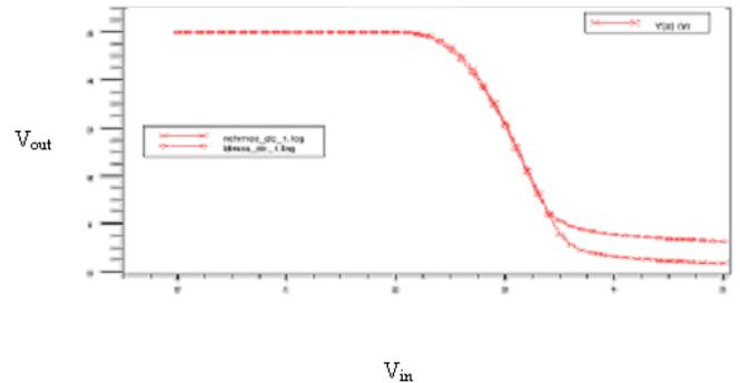
**Fig. 8:** Inverter output in DC analysis
