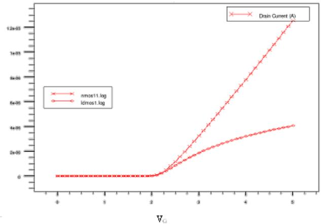
**Fig. 2b:** Drain characteristics ( $V_{GS}$  vs  $I_D$ ).
