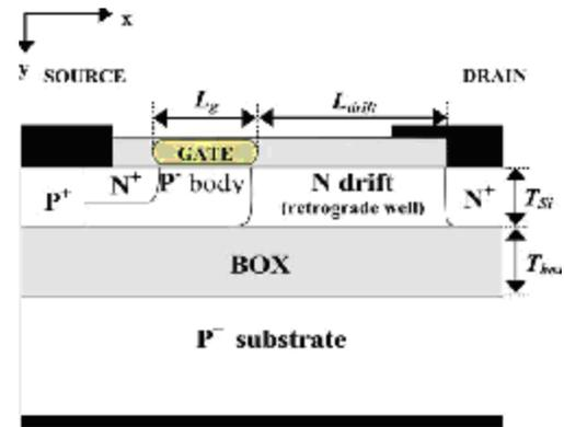
Fig. 1: Cross-section of a 38V LDMOS transistor.
