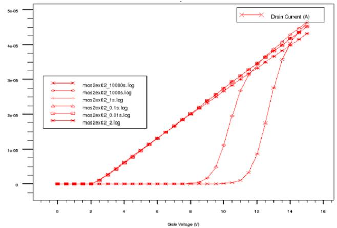
**Fig. 14:** Hot electron effect on MOSFET showing drastic change on threshold voltage.
