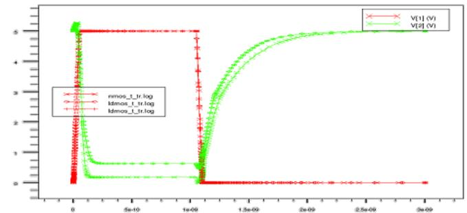
Fig. 6: Transient Analysis of Inverter circuit
