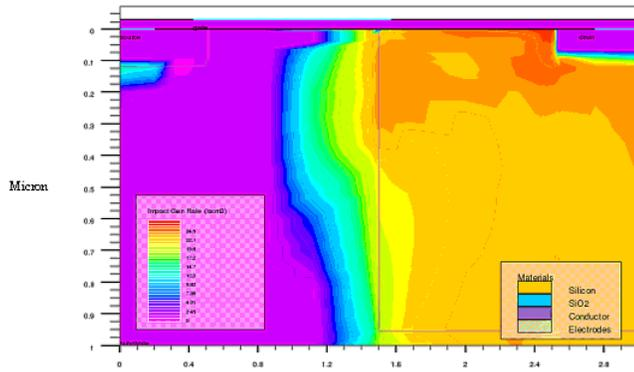
Fig. 15: Impact ionization at  $n\text{-drift}=1.1\text{e-}16$ .
