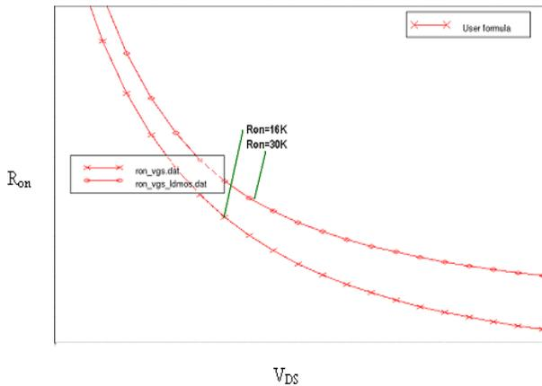
**Fig2a:**  $R_{on}$  vs.  $V_{DS}$  for n-MOS and LDMOS.
