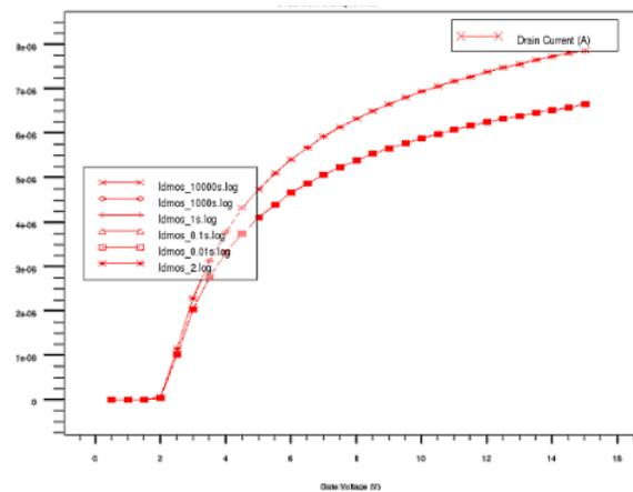
**Fig. 13:** Hot electron effect on LDMOSFET showing minimal change on threshold voltage.
