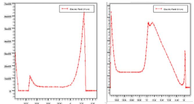
Fig. 5: Electric Field distribution for n-MOS and LDMOS.
