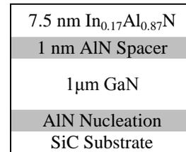
**Figure 2:** 100-nm gate-InAlN/GaN HEMT with AlN interlayer as spacer and nucleation. The growth direction is along z-axis.
