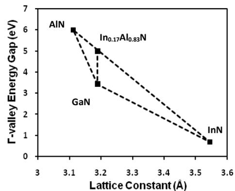
**Figure 1:** Variation of Energy Bandgap with Lattice Constant for (Al,In)GaN based heterostructure matrix.
