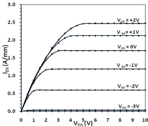
**Figure 3:** Simulated Drain current characteristics of proposed HEMT measured from  $V_{GS} = -3 V$  to  $+2 V$ , in steps of  $+1 V$ .
