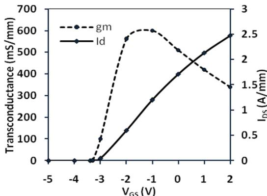
**Figure 4:** Transfer characteristics of simulated structure showing a maximum transconductance of 600 mS/mm.
