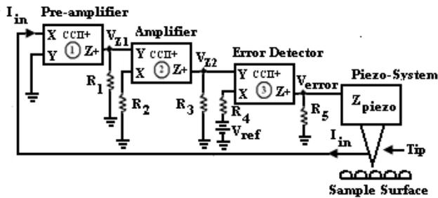
Figure 3. Proposed feedback Circuit along with Piezo - System
