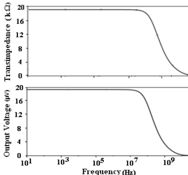
Figure. 4. Transimpedance and output voltage of the pre-amplifier with  $I_{in} = 1$ nA and  $R_1= 20$ k $\Omega$
