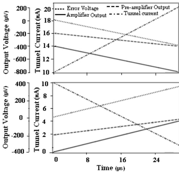
Figure 6. Input tunnel current and corresponding output voltage of pre-amplifier, amplifier and error detector
