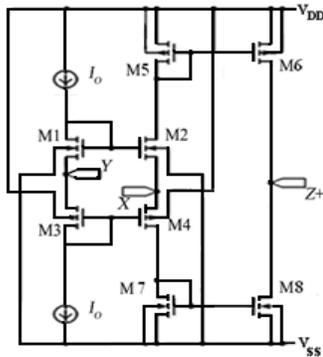
Figure 2. Internal structure of CCII+
