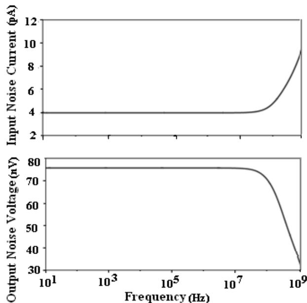
Figure 5. Input noise current and Output noise voltage of the pre-amplifier
