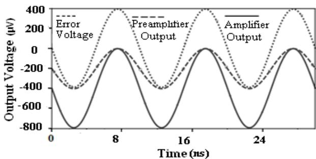
Figure 8. Output of pre-amplifier, amplifier and error detector
