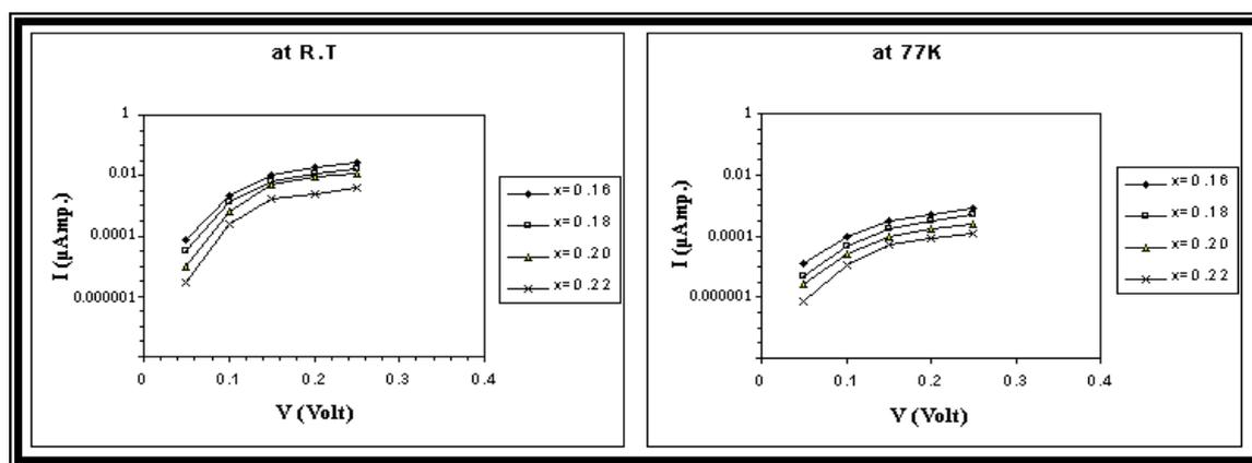
**Figure 4:** I-V characteristics at forward bias voltage on semilogarithm scale for  $Hg_{1-x}Cd_xTe/Si$  diodes of different Cd content at (a) R.T and (b) 77 K.
