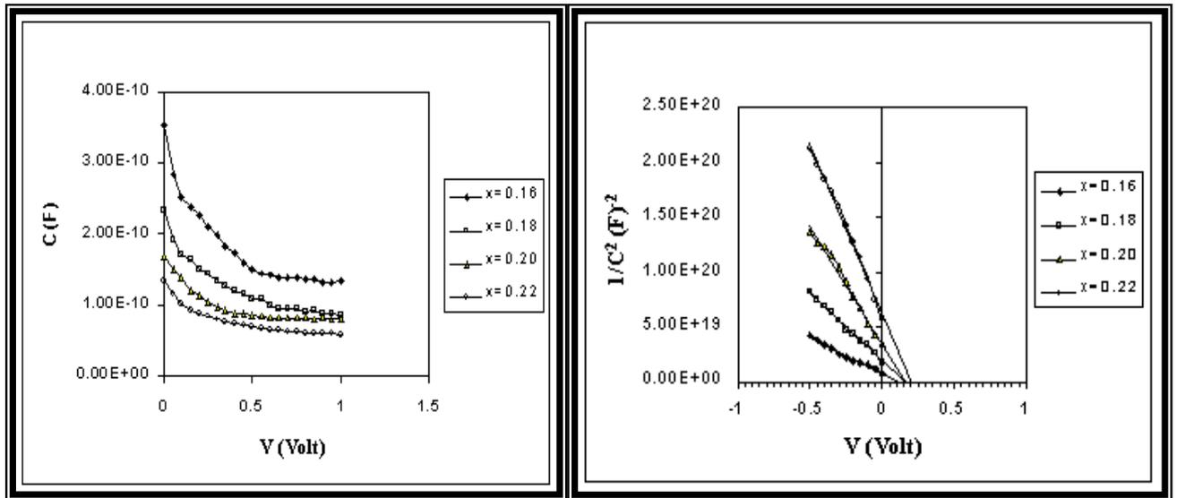
**Figure 1:** Capacitance vs. reverse applied voltage for Hg<sub>1-x</sub>Cd<sub>x</sub>Te/Si diodes of different Cd content.
