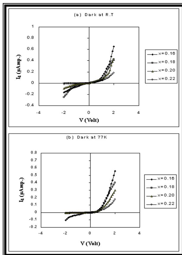
**Figure 3:** I-V Characteristics for  $Hg_{1-x}Cd_xTe/Si$  diodes at forward and reverse bias voltage of different Cd content at (a) R.T and (b) 77 K.
