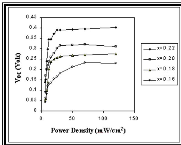
**Figure 7:** The variation of  $V_{oc}$  as a function of power intensity for  $Hg_{1-x}Cd_xTe/Si$  diodes of different Cd content.
