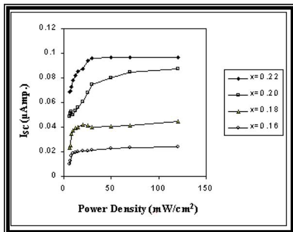
**Figure 6:** The variation of  $I_{sc}$  as a function of power intensity for  $Hg_{1-x}Cd_xTe/Si$  diodes of different Cd content.
