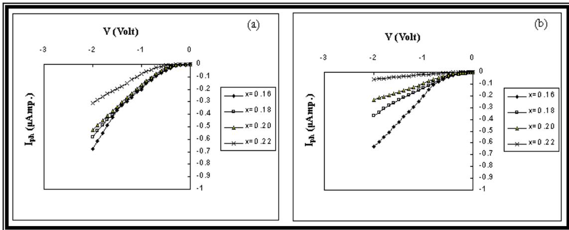
**Figure 5:** The relation between  $I_{ph}$  and reverse bias voltage for  $Hg_{1-x}Cd_xTe/Si$  diodes of different Cd content at (a) R.T and (b) 77 K.
