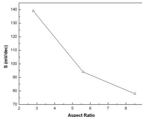
**Figure 9:**  $V_T$ ,  $I_{ON} / I_{OFF}$ , DIBL and S as a function of aspect ratio
