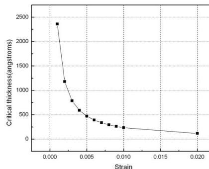
Figure 3(a): lattice constant variation along the <100> growth direction **Figure 3(b):** Schematic of strained heterolayer epitaxy **Figure 3(c):** Mathews and Blacklesse critical thickness model
