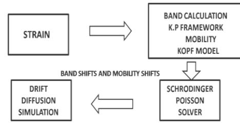
**Figure 4:** Simulation flow for strain modeling
