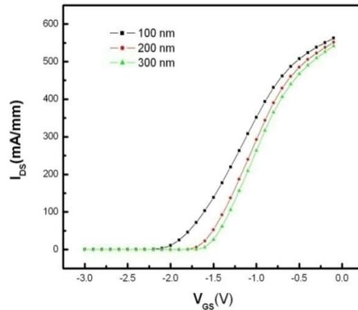
**Figure 8:** Comparison of transfer characteristics for different gate lengths
