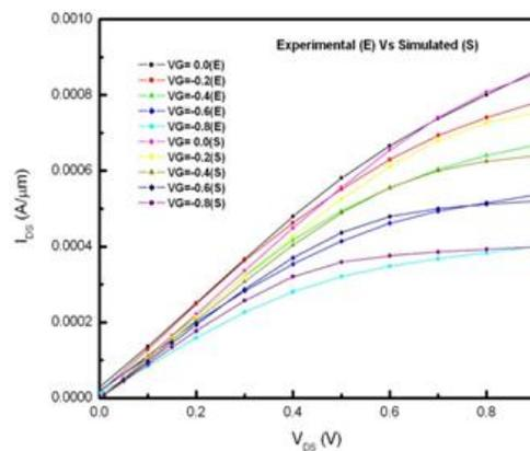
**Figure 5:** Comparison of output characteristics of simulated and investigational 300 nm device
