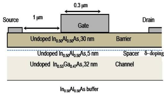
Figure 2: Schematic of 300 nm HEMT
