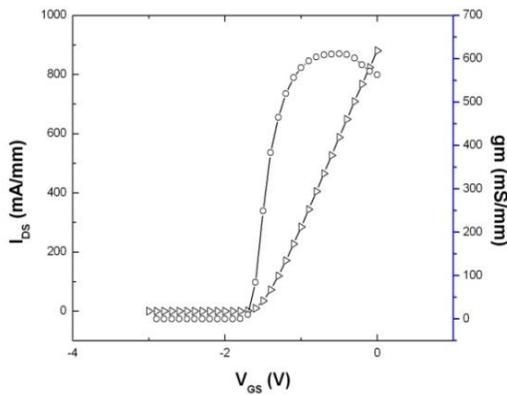
**Figure 6:** Simulated transconductance and transfer characteristics for 300 nm HEMT
