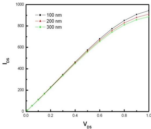
**Figure 7:** Comparison of drain characteristics for different gate lengths
