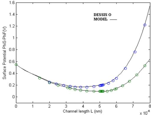
Figure 10 Plots for different values of  $V_{DS}=1V, 0.1V$  with  $N_p=1.2 \times 10^{18}, N_a=1 \times 10^{17} \text{ cm}^{-3}$  against the applied voltages  $V_{GS}=0V = V_{GB} = V_{SB}, L=80 \text{ nm}$ .
