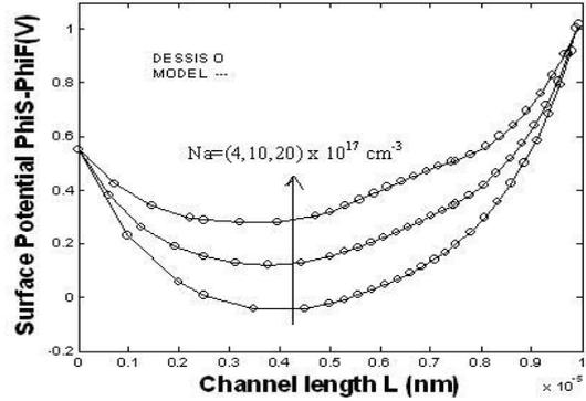
Figure 17 The plots for three different values of the substrate doping  $N_a = 4 \times 10^{17}$ ,  $10^{18}$  and  $2 \times 10^{18} \text{ cm}^{-3}$  against the applied voltages  $V_{GS} = 0V$  and  $V_{DS} = 0.5V$  for SHDMG.
