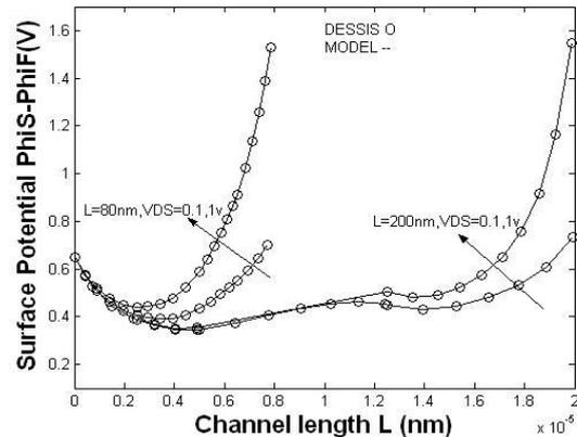
Figure 18 The variation of the potential profiles in an SHDMG device with two different channel lengths  $L = 80$  and  $200 \text{ nm}$  for  $N_a = 6 \times 10^{17} \text{ cm}^{-3}$  against two different drain voltages  $V_{DS} = 0.1V$  and  $1V$  along with  $V_{SB} = 0.1V$  and  $V_{GB} = 0.2V$ .
