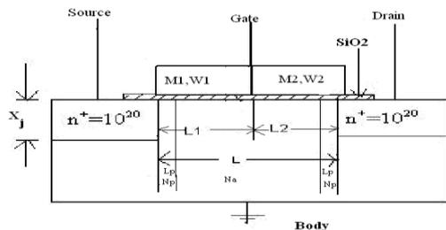
Figure 1 An n-channel Double pocket DMG-MOSFET structure.
