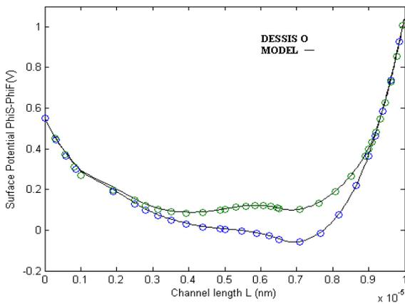
Figure 11 The potential profiles for two sets of gate materials  $W_1=4.3$  and  $W_2=4.1$  and  $W_1=4.2$  and  $W_2=3.9$  for  $L=100 \text{ nm}, N_p=2 \times 10^{18}, N_a=1 \times 10^{17} \text{ cm}^{-3}$  against the applied voltages  $V_{GS}=0V = V_{GB} = V_{SB}, V_{DS}=0.5V$ .
