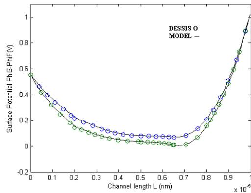
Figure 8 The plots for two different values of the pocket doping  $N_p=1.2 \times 10^{18}$  and  $1.8 \times 10^{18} \text{ cm}^{-3}$  against the applied voltages  $V_{GS}=0 \text{ V} = V_{GB} = V_{SB}$  and  $V_{DS}=0.5 \text{ V}$ ,  $N_a=1 \times 10^{17} \text{ cm}^{-3}$ .
