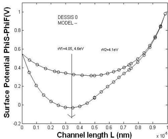
Figure 19 The SHDMG potential profiles for a fixed value of  $W_2=4.1$  eV, with two different values of  $W_1=4.05$  and  $4.6$  eV, respectively.
