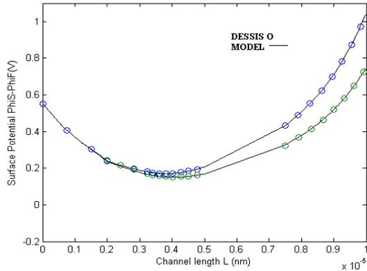
Figure 15 The plots for two different values of  $V_{DS} = 0.5V$  and  $2V$ , considering  $N_p = 1.2 \times 10^{18}$ ,  $N_a = 1 \times 10^{17} \text{ cm}^{-3}$  against the applied voltages  $V_{GS} = 0V = V_{GB} = V_{SB}$ ,  $L = 100 \text{ nm}$ .
