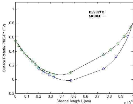
Figure 16 The potential profiles for two sets of gate materials  $W_1 = 4.25$  and  $W_2 = 4.1$  and  $W_1 = 4.2$  and  $W_2 = 3.76$  for  $L = 100 \text{ nm}$ ,  $N_p = 1.2 \times 10^{18}$ ,  $N_a = 4 \times 10^{17} \text{ cm}^{-3}$  against the applied voltages  $V_{GS} = 0V = V_{GB} = V_{SB}$ ,  $V_{DS} = 0.25V$ .
