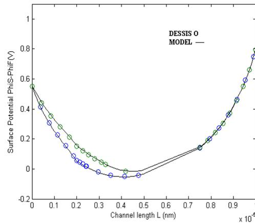
Figure 14 The plots for two different values of the pocket doping  $N_p=2.2 \times 10^{18}$  and  $1.2 \times 10^{18} \text{ cm}^{-3}$  against the applied voltages  $V_{GS}=0V = V_{GB} = V_{SB}$  and  $V_{DS}=0.25V, N_a=4 \times 10^{17} \text{ cm}^{-3}$
