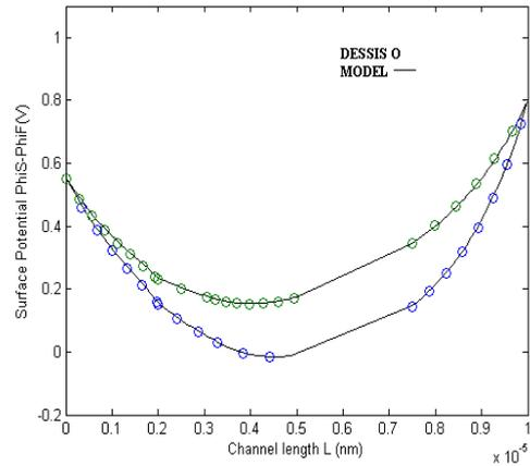
Figure 13 The plots for two different values of the substrate doping  $N_a=4 \times 10^{17}$  and  $1 \times 10^{17} \text{ cm}^{-3}$  against the applied voltages  $V_{GS}=0V = V_{GB} = V_{SB}$  and  $V_{DS}=0.25V$ .
