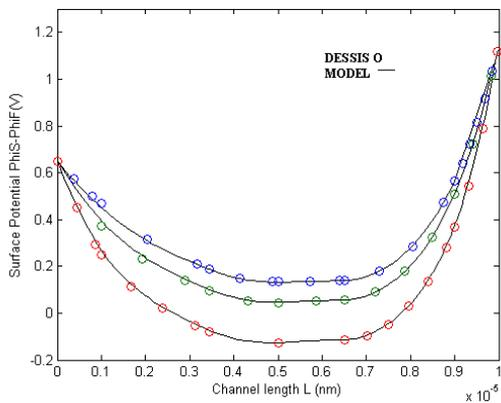
Figure 12 The potential profiles for three sets of gate bias a)  $V_{GS}=0.1V, V_{GB}=0.2V, V_{SB}=0.1V$  b)  $V_{GS}=0V, V_{GB}=0.1V, V_{SB}=0.1V$  c)  $V_{GS}=-0.2V, V_{GB}=-0.1V, V_{SB}=0V$  for  $L=100 \text{ nm}, N_p=1.2 \times 10^{18}, N_a=4 \times 10^{17} \text{ cm}^{-3}, V_{DS}=0.5V$ .
