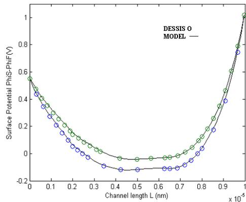
Figure 9 The plots for two different values of the substrate and pocket doping  $N_p=1.8 \times 10^{18}$ ,  $N_a=6 \times 10^{17} \text{ cm}^{-3}$  and  $N_p=1.2 \times 10^{18}$ ,  $N_a=4 \times 10^{17} \text{ cm}^{-3}$  against the applied voltages  $V_{GS}=0 \text{ V} = V_{GB} = V_{SB}$  and  $V_{DS}=0.5 \text{ V}$ .
