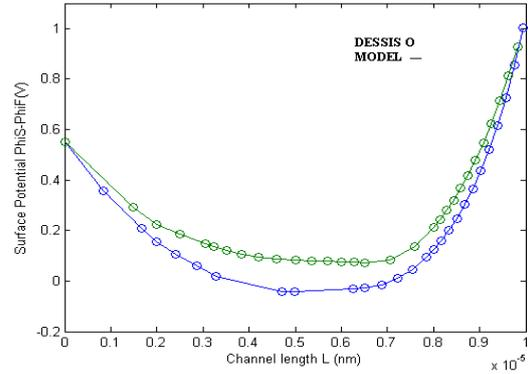
Figure 7 The plots for two different values of the substrate doping  $N_a=4 \times 10^{17}$  and  $1 \times 10^{17} \text{ cm}^{-3}$  against the applied voltages  $V_{GS}=0 \text{ V} = V_{GB} = V_{SB}$  and  $V_{DS}=0.5 \text{ V}$ .
