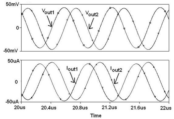
**Figure 11** Simulated output voltage and current waveforms at 1.59MHz
