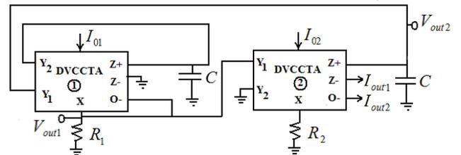
Figure 4 Proposed voltage mode and current mode quadrature oscillator
