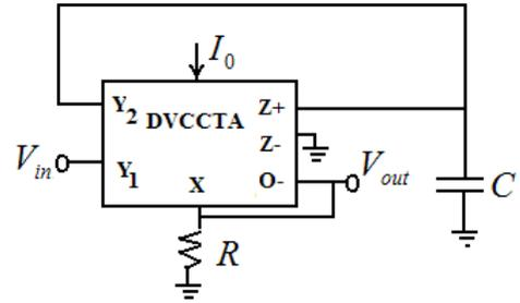
Figure 3 Proposed voltage mode all pass filter
