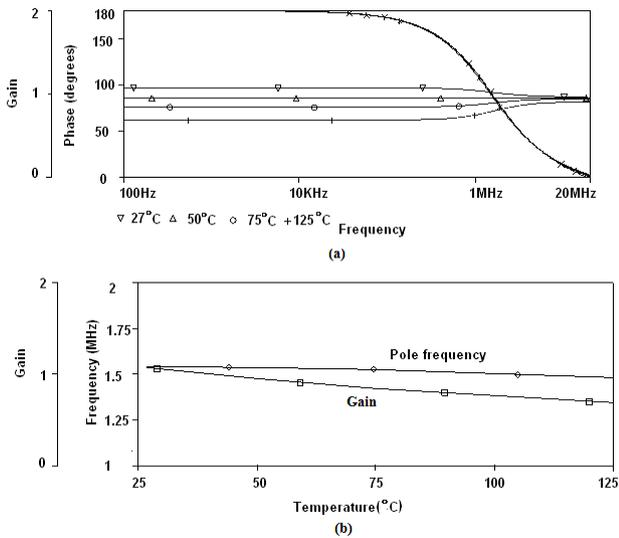
**Figure 10** Effect of temperature on all pass response (a) frequency vs phase and gain at different temperatures (b) temperature vs gain at 100 Hz and pole frequency.
