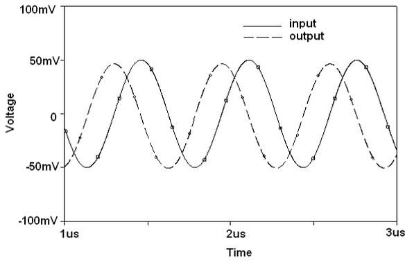
**Figure 8** Transient response of the filter with sinusoidal input at 1.59MHz
