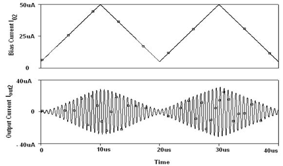
**Figure 12** The amplitude modulated waveform for  $I_{out2}$  for various values of  $I_{02}$
