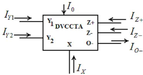
Figure 1. Circuit symbol of DVCCTA
