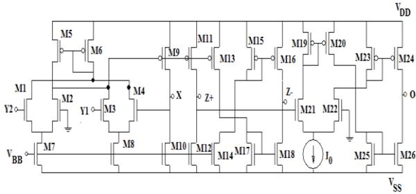
Figure 2. Internal structure of DVCCTA using CMOS
