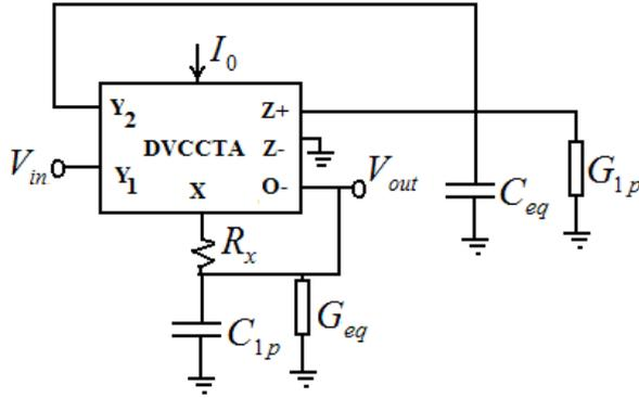
Figure 5 Proposed all pass filter with parasitic components
