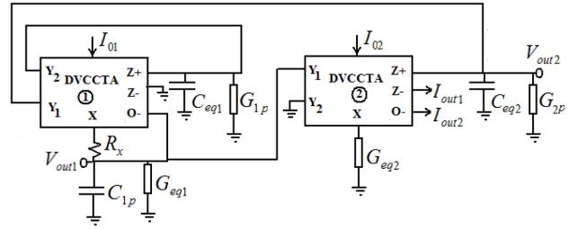
Figure 6 Proposed quadrature oscillator with parasitic components
