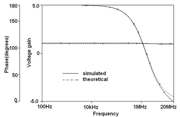
Figure 7 Magnitude and phase response of the proposed voltage mode all pass filter
