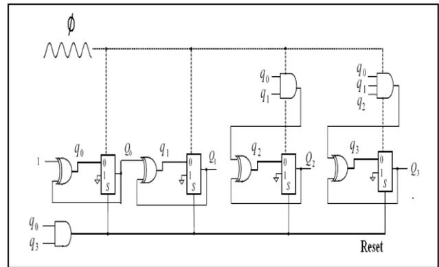
Figure 9. Schematics of decimal up counter based on EEAL logic
