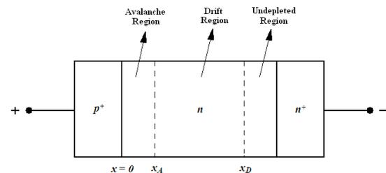
Figure 1: Schematic of a reverse biased flat SDR.
