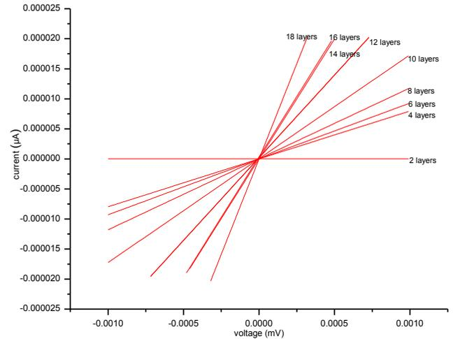
**Figure 3:** I-V characteristic for multilayer TiO<sub>2</sub> nanocoated glass substrate.
