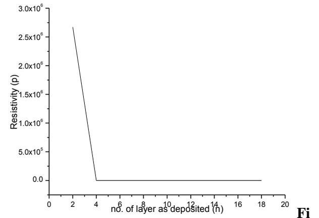
**Figure 4:** Resistivity of TiO<sub>2</sub> nanocoated glass substrate at different number of layer.
