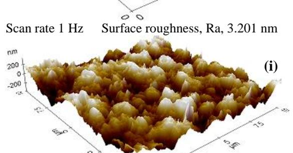
**Figure 2:** Three-dimensional imaging of multilayer TiO<sub>2</sub> nanocoated glass: (a) 2 layers, (b) 4 layers, (c) 6 layers, (d) 8 layers, (e) 10 layers, (f) 12 layers, (g) 14 layers, (h) 16 layers and (i) 18 layers.
